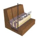
Spread 25mm of washed sand over the compacted base.
